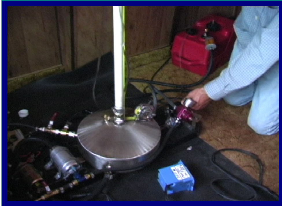
JPEG 3 - Fuel usage measuring rig as installed in the Champion 440 RV. The test engineer is shown setting up the rig.
