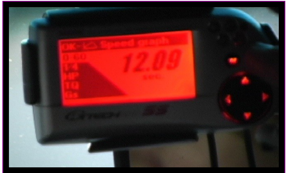
JPEG 7 : Windscreen mounted accelerometer - showing the 0 to 60 times. As recorded by the onboard video camera.
