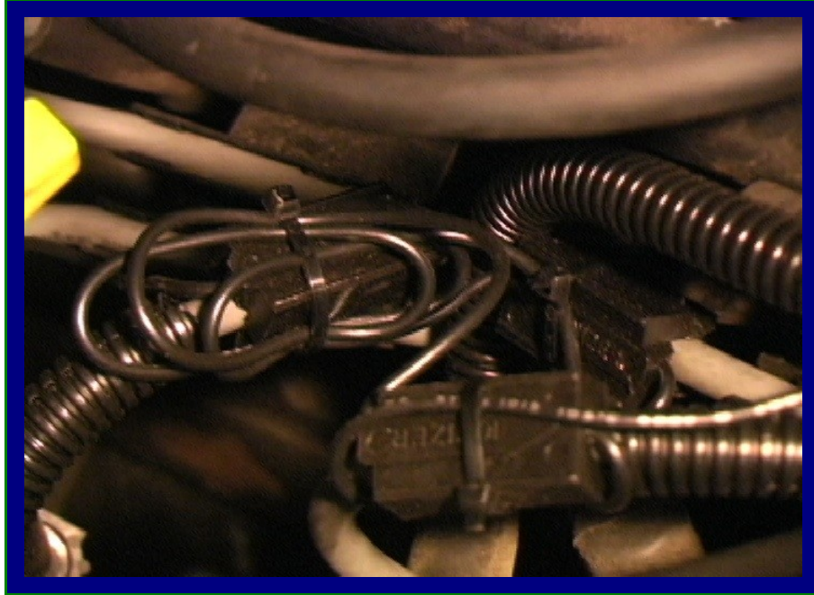
JPEG 1 - Ionizer Blocks installed on the JEEP Cherokee. Note the "split-loom" and the looped connecting-wire layout.
