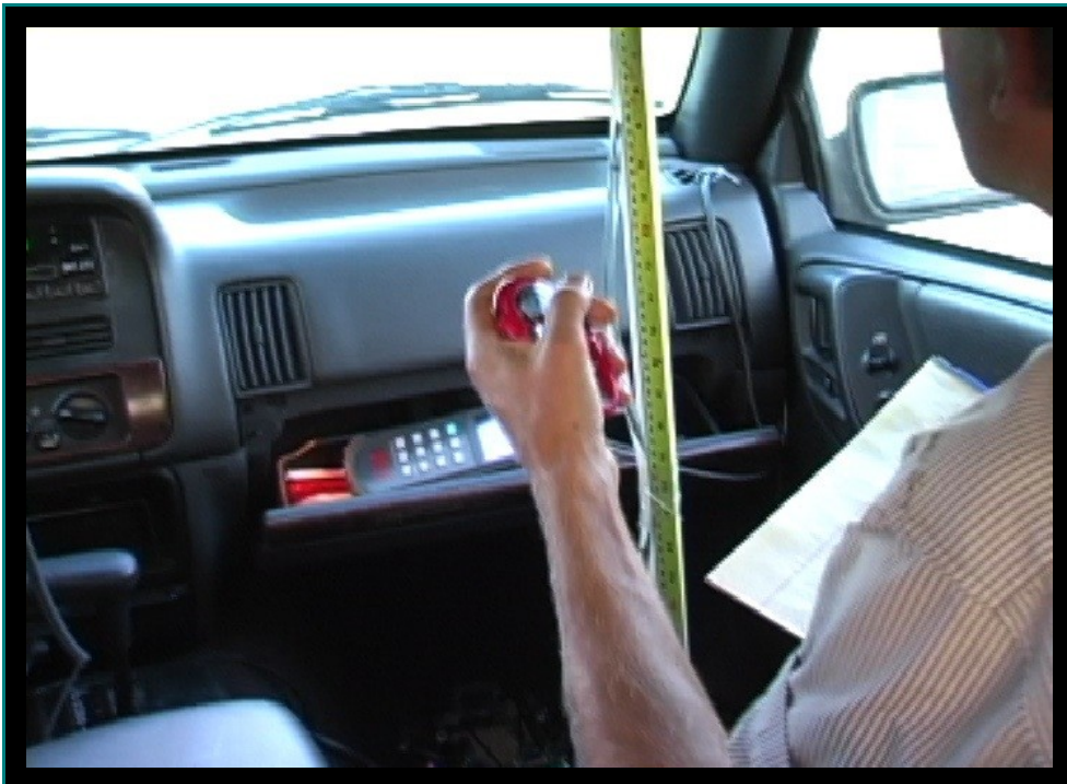
JPEG 4 : The test engineer captures the fuel usage and the elapsed time readings. All tests are fixed-course road runs.
